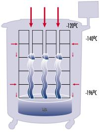
Heat path into standard LN2 refrigerator in vapor phase mode fitted with vapor sleeve. Note additional heat path into liquid reservoir provided by sleeve.
