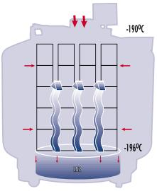
MVE-190HE system in vapor mode. Note that only internal heat paths are created to improve the temperature gradient giving - 190°C below the lid.
